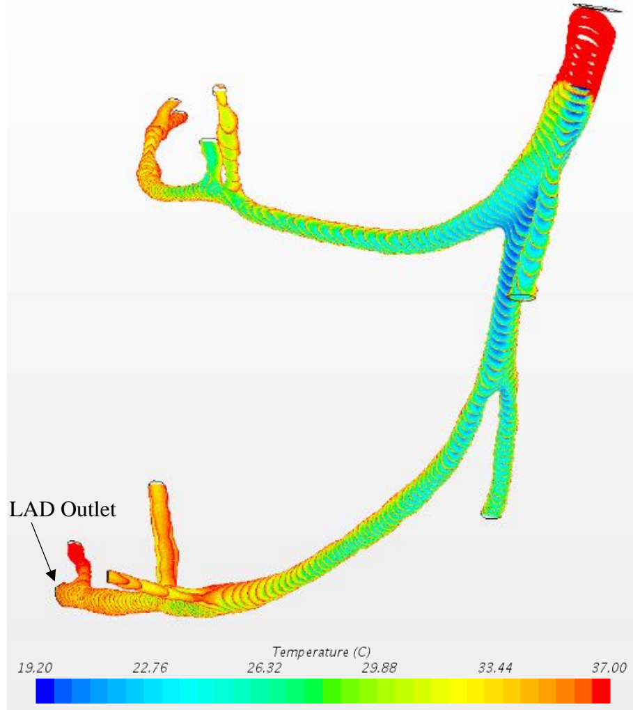
Figure 7.37. Structural-thermal relationship in HH102 LAD for 68.85 ml/min guide extension flow rate. Note: proximal guide extension inlet temperature is 19.2°C, and LAD outlet temperature is 30.47°C.
